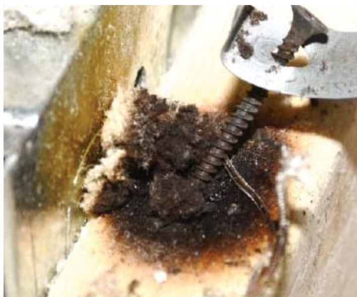
Figure 10 – Photograph of the thermal damage, evidence of combustion, and consumption of the wood and cellulosic insulation taken after the end of the second test.
