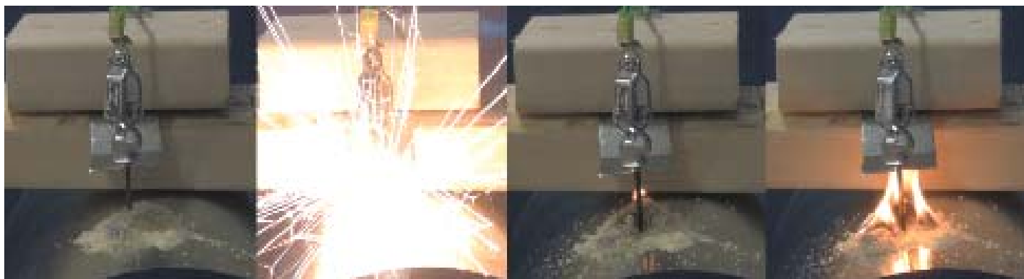
Figure 5 – Still images taken during Test Number 1 with no added resistance and no grounding of the HVAC duct.
