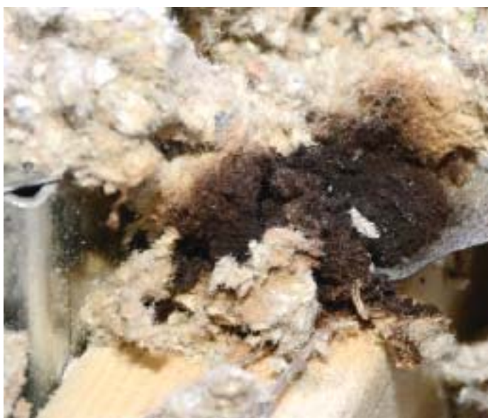
Figure 10 – Photograph of the thermal damage, evidence of combustion, and consumption of the wood and cellulosic insulation taken after the end of the second test.
